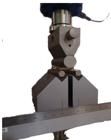
Plate 2. Three-point bending technique of bone breaking
