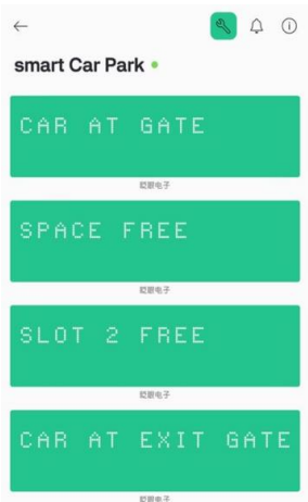
Fig. 6. Visualization Through Blynk IoT Mobile App
