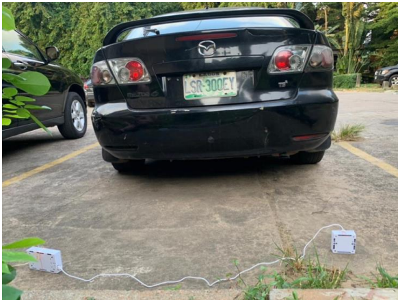
Fig. 5. The integrated sensor setup for a parking spot
