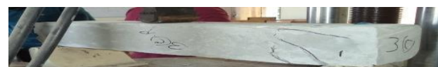
Fig. 10(e). Failure mode for reinforced concrete beam sample cast with F5R5S10 (Siddika et al. , 2021).
