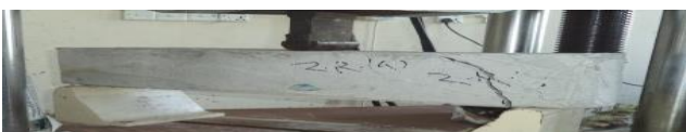
Fig. 10(c). Failure mode for reinforced concrete beam sample cast with F10R5S0 (Siddika et al. , 2021).
