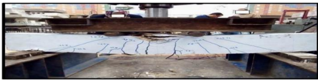
Fig. 14. Sample of cracks propagation and failure mode (El-Sayed et al., 2019).
