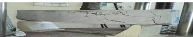
Fig. 10(b). Failure mode for reinforced concrete beam sample cast with F5R10S0 (Siddika et al. , 2021).
