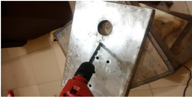
Fig. 1. Drilling of Metallic Sheet for top cover of the aspirator casing
