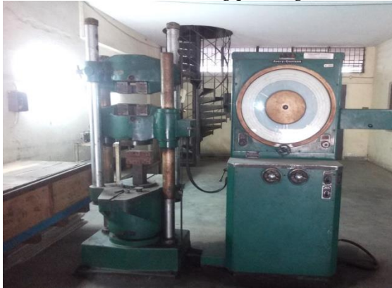
Figure 6: Die placed on Axial Loading Machine
