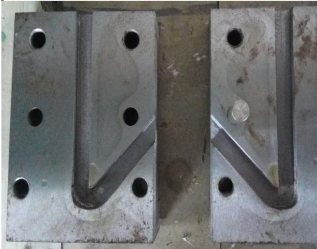
Figure 2: Die with 45° Extrusion Angle
