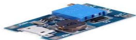
Figure 3: DC-DC Boost converter
