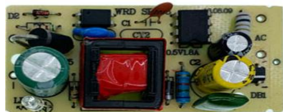
Figure 2.0 AC to DC converter
