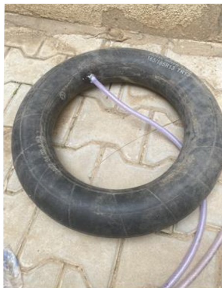
Figure 3: Produced gas is stored in the tube.
