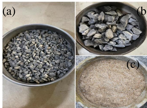
Fig. 2. Aggregates used for the experiment (a) sample \frac{3}{4} of coarse aggregates (b) sample of \frac{5}{8} coarse aggregates (c) fine aggregates
