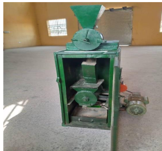
Figure 2: Pictorial view of the domestic waste comminution and drying machine
