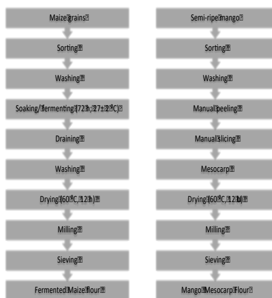
Fig. 1: Flowchart for production of fermented maize flour and mango mesocarp flour
