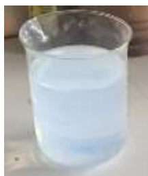
Fig. 1: 5g of silver nanoparticle in solution of 100ml of distilled water
