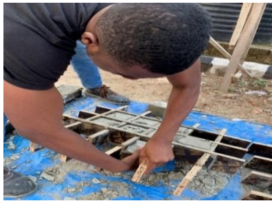
Fig. 2: Demoulding of concrete cubes
