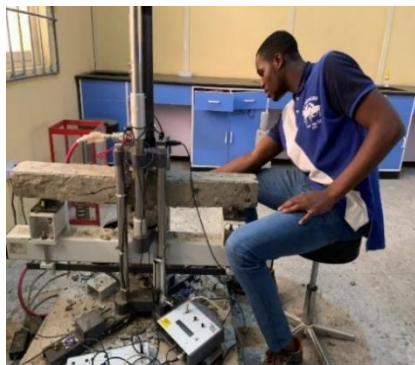
Fig. 4: Flexural test using the ASTM 293 C
