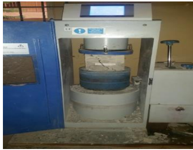
Fig. 1: Compression Testing Machine in action
