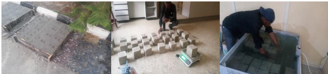
Fig. 3: Casting, de-molding and curing of concrete cubes
