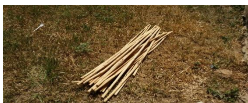
Fig. 1: Rattan cane or sticks used as Reinforcement
