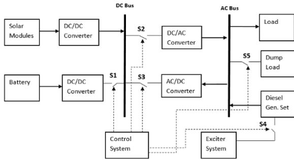
Fig. 4. Modelled Block Diagram of Proposed Off-grid Hybrid Microgrid Power System with Scheduling (Control) System.
