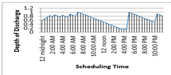
(c) Battery Depth of Discharge during scheduling
