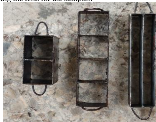
Fig. 2: Metal moulds for moulding the biocomposites
