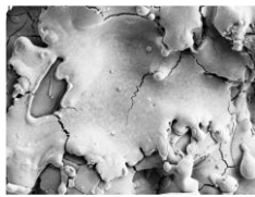
Fig. 2: The surface of an APS YSZ coating, showing how a molten particle has flattened on impact
