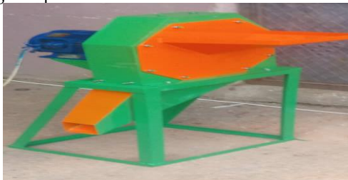
Fig. 4: The Designed and Fabricated Hammer Mill
