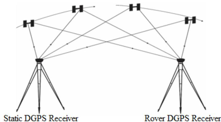
Figure 1: Arrangement of rapid static GNSS method of observations
