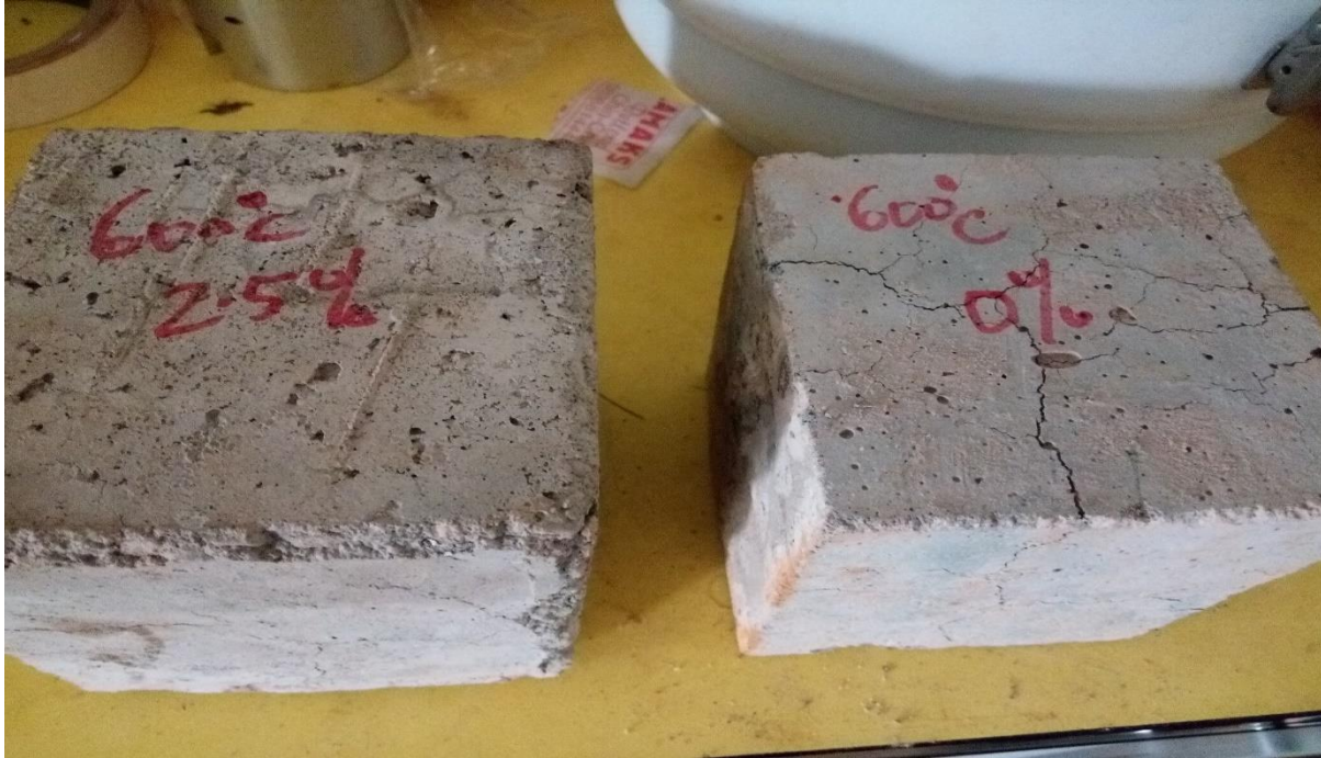
Plate 2: Spalling Effect on control samples at 600°C compared to HDPE samples
