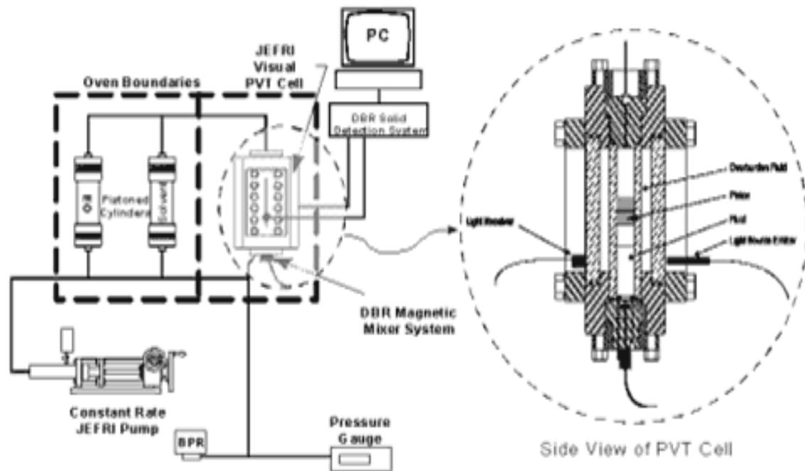
**Figure 3: Schematic Diagram of Schlumberger PVT Cell Equipped with Solid Detection System (SDS) (Schlumberger, 2015)**
