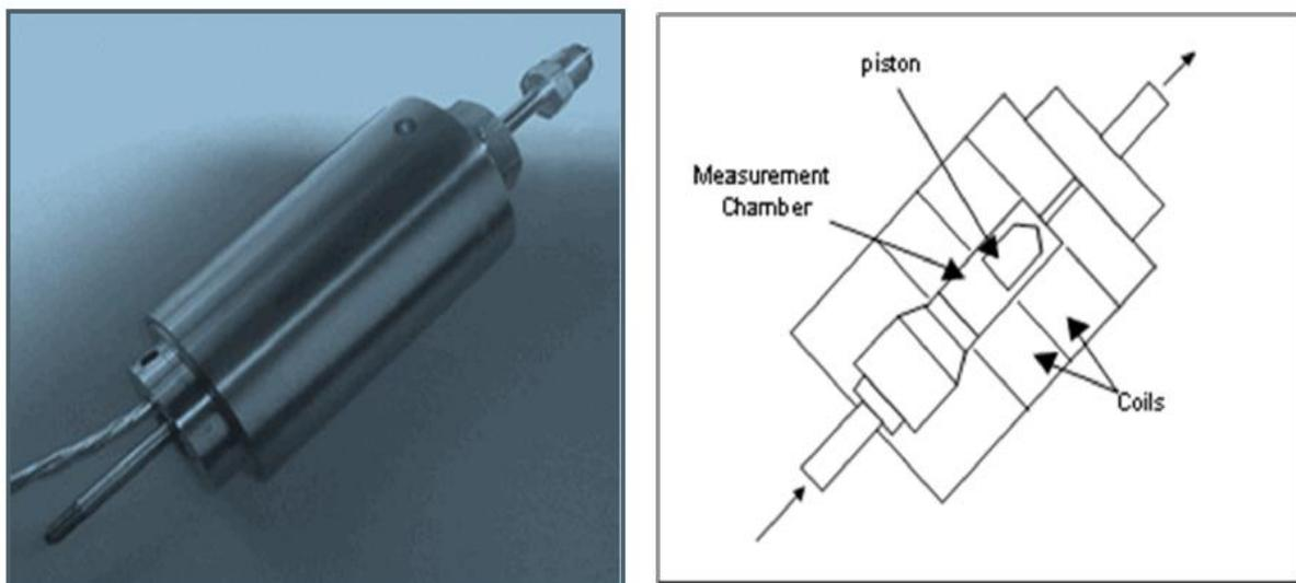
**Figure 4: Schematic Diagram of Cambridge Electromagnetic Viscometer (Schlumberger, 2015).**
