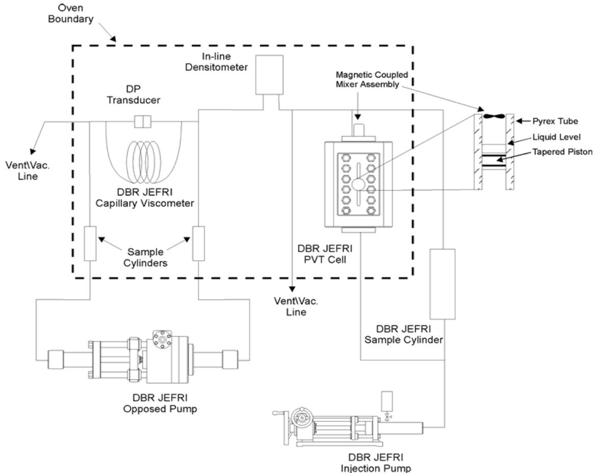
Figure 5: Schematic of Capillary Viscometer Setup (Schlumberger, 2015)
