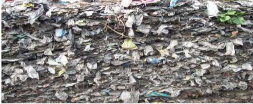
Figure 1. View of a 2 m profile of the ground occupied by thermoplastic waste in Kinshasa/Lingwala
