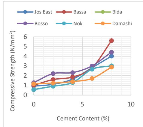
**Figure 8: Comparative Compressive Strength at 28days of CEB**
