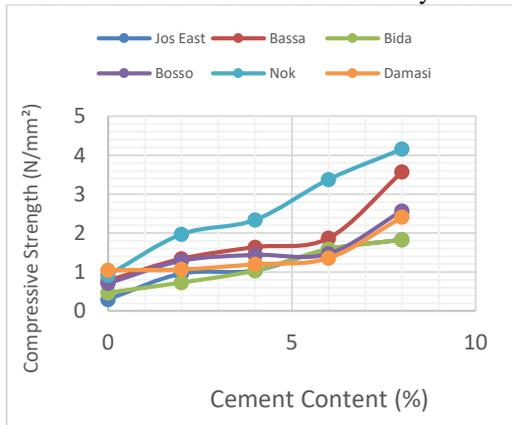
**Figure 7: Comparative Compressive Strength at 7days of CEB**
