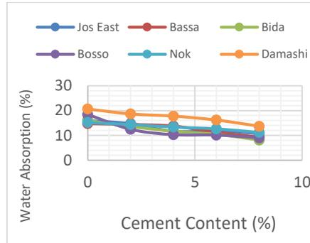
**Figure 6: Water absorption test of the soil samples**
