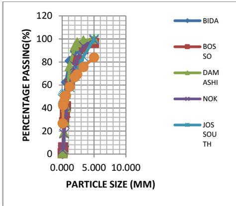
Figure 3: Sieve Analysis of the soil samples
