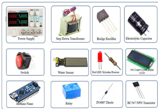
Figure 4.1: Components of the proposed Intelligent Irrigation System
