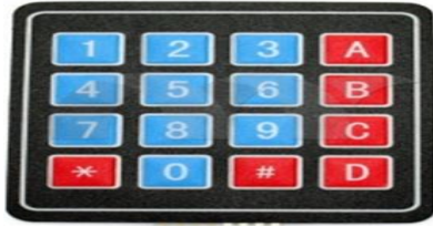
Figure 2.4g: 4 X 4 Matrix Keypad
