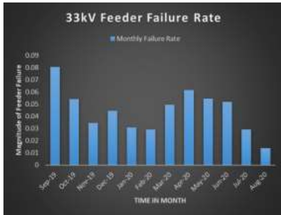
Figure 3.1: Monthly Failure Profile of 33 kV Feeder of Ugbowo 2x15 MVA, 33/11 kV Injection Substation.
