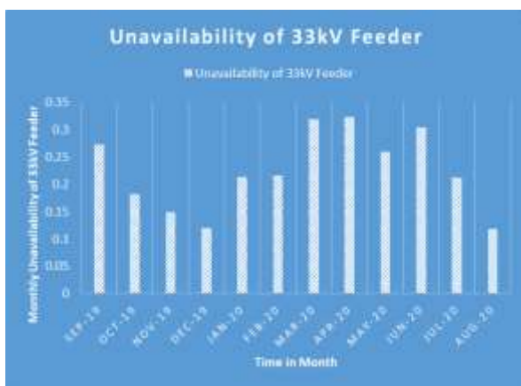
Figure 3.7: Monthly Unavailability of 33 kV Feeder of Ugbowo 2 x 15 MVA, 33/11 kV Injection Substation.
