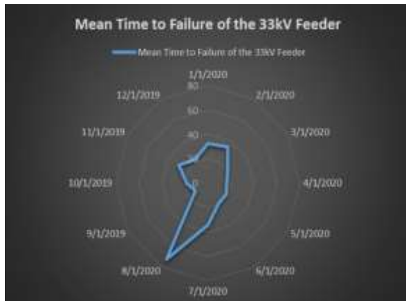
Figure 3.5: Monthly Mean Time to Failure of the 33 kV Feeder of Ugbowo 2x15 MVA, 33/11 kV Injection Substation.
