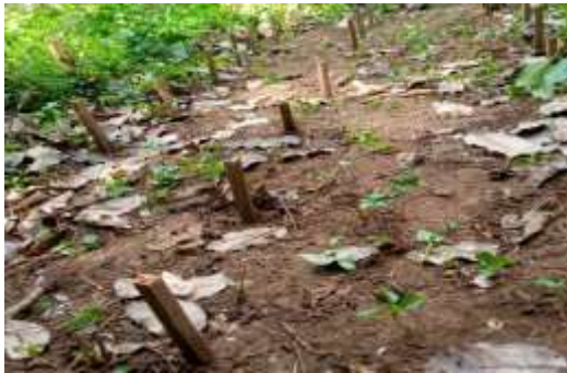
Plate 3.1: Wood samples of Boscia angustifolia and Ceiba petandra (reference species) at Graveyard.
