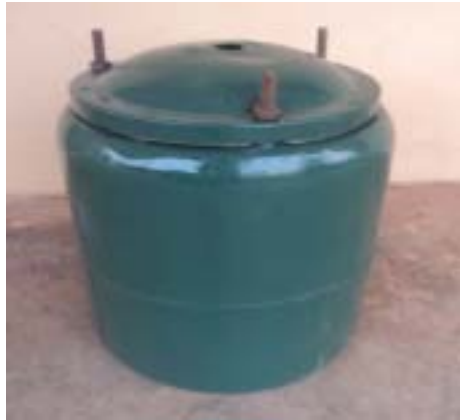
Fig. 6: The Finished Grinding Chamber (jar)
