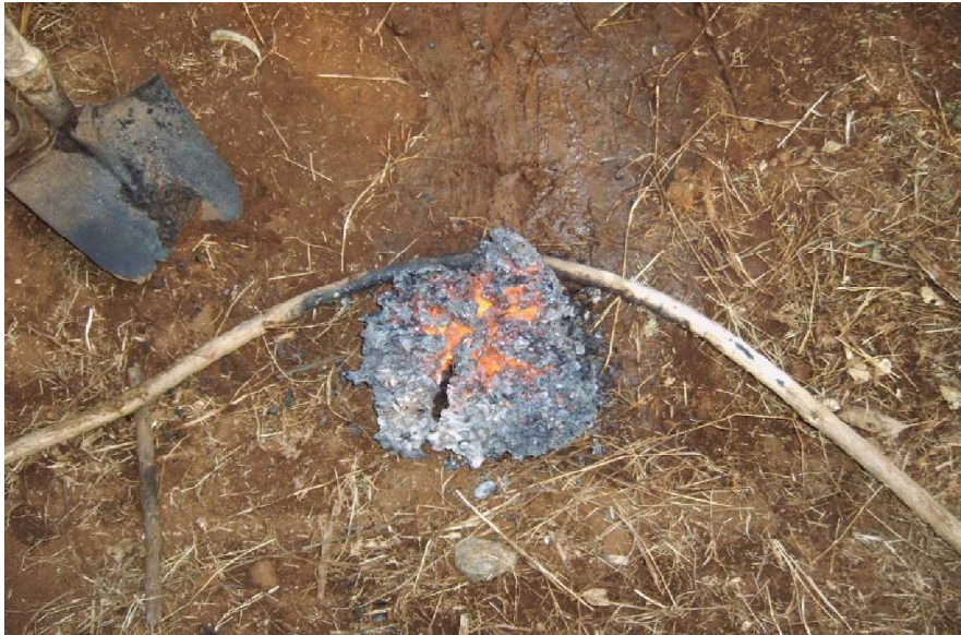
Fig.8: a dragged bloom leaving marks on the ground, still glowing
