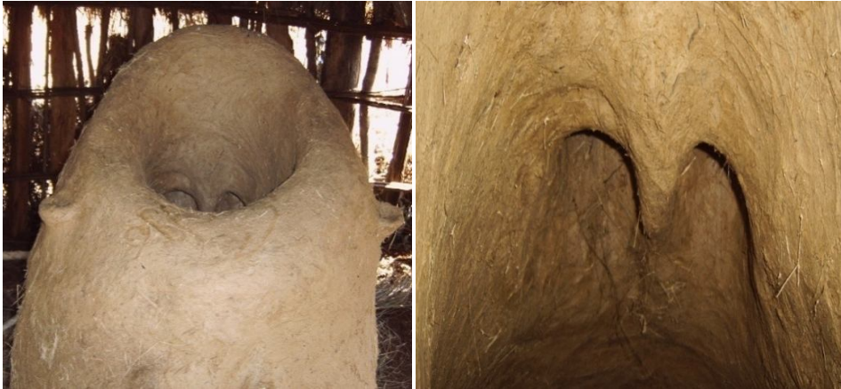
Fig.3: upper part of the furnace head and ear like structure (left) and zoomed-in epiglottis (right)
