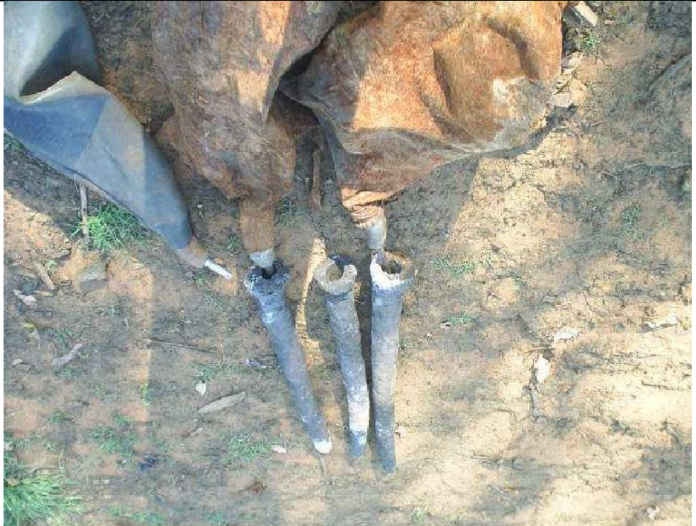
Fig.5: the three components of tuyères and the bag bellows
