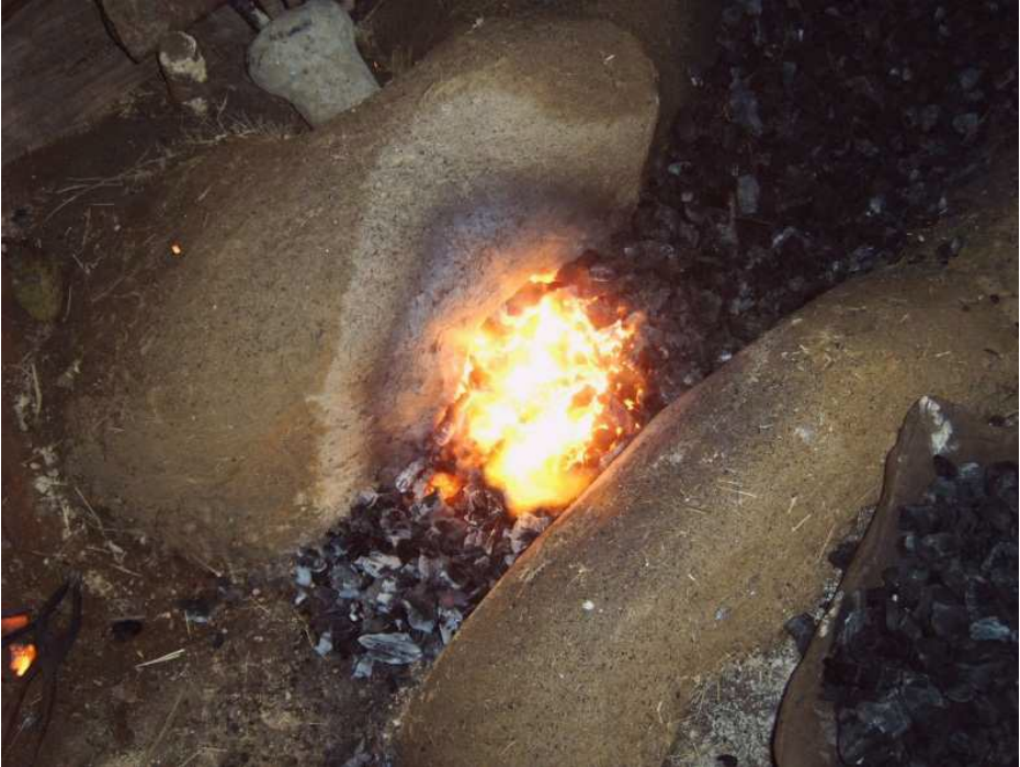
Fig.9: bloom at bubbling stage in the smithing forges in southwest Wollega
