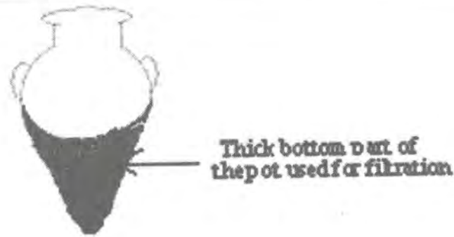
Figure 1 Conical clay pot fluoride filter made with different sand to clay ratios
