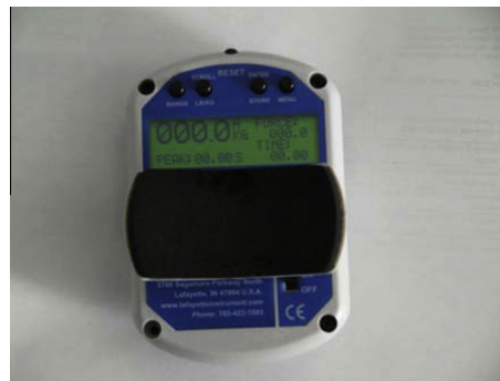
Figure 1 Lafayette Manual Muscle Test System (Model 01163, Lafayette Instrument Company, Lafayette, IN, USA).
