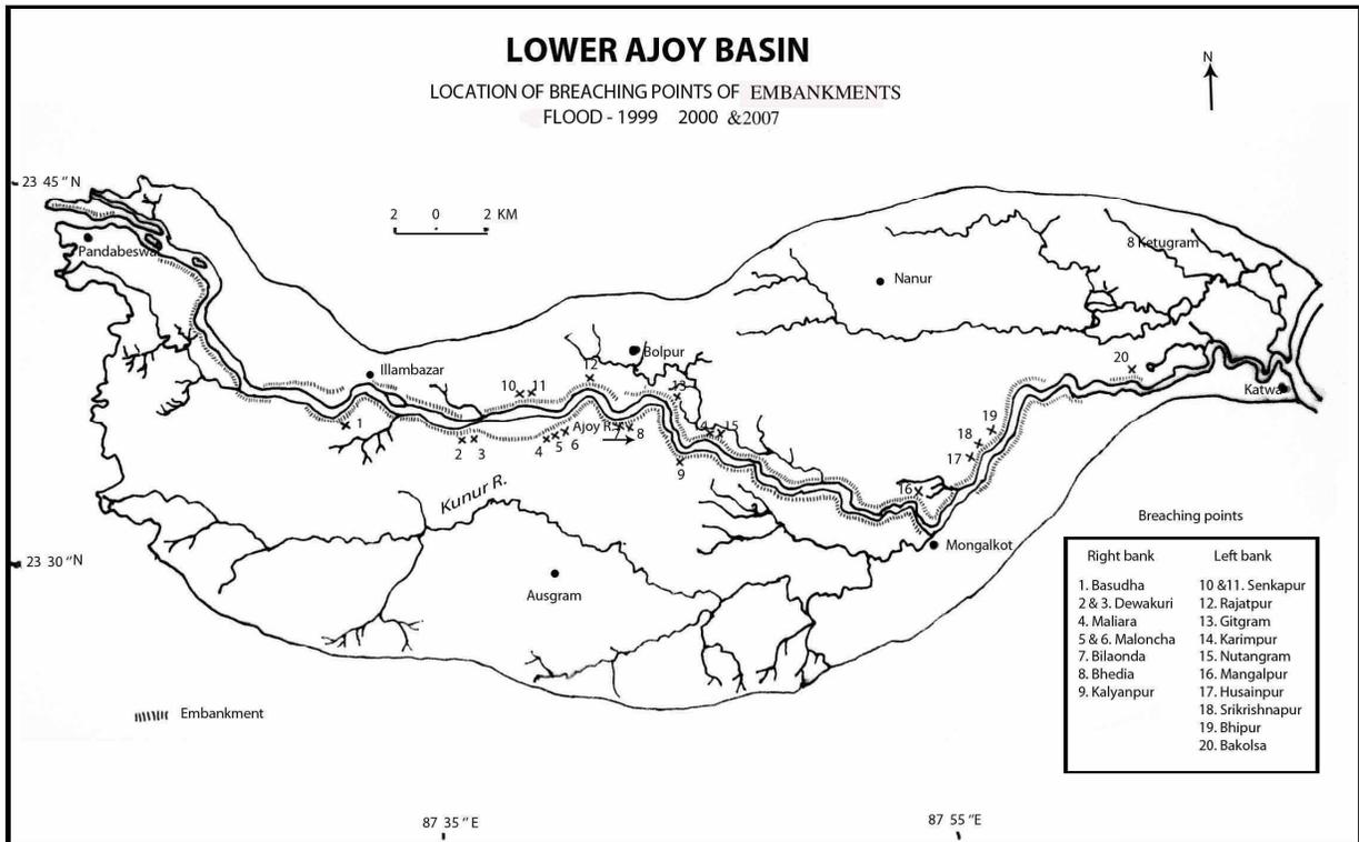
Figure 3 Breaching Points of Embankments
