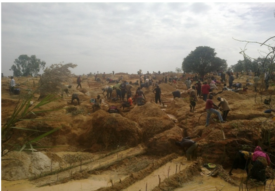
Plate 1: Tin separation using ground Sluice Boxes
