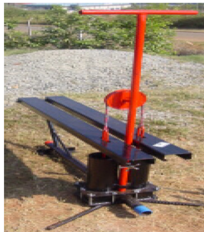
Figure 1: A metal treadle pump: (a) pictorial view and (b) isometric projection.
