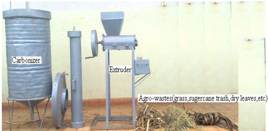
Fig.1. Carbonizer, Extruder and agro-wastes (grass, sugarcane trash, coffee husk, dry leaves, etc.)
