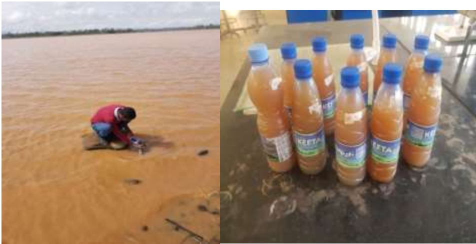
Fig. 2. In-situ measurement of physicochemical properties and water sampling for nutrient analysis in Koga Reservoir.
