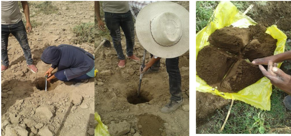
Fig. 3. Soil sampling techniques at different depths.
