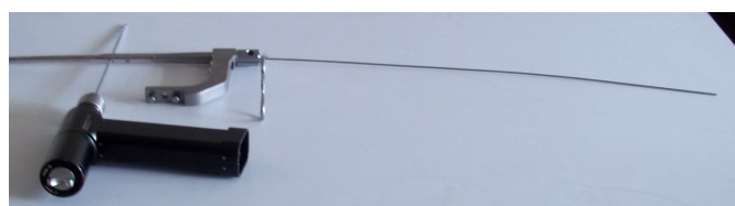
Figure 13: A clamp is used to mark out the length of guide wire that went into the nail
