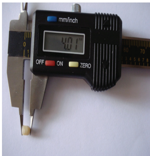
Figure 5 The Electronic Digital Vernier Caliper used to measure the DOC with a specimen in situ
