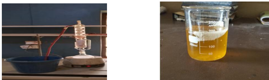
Figure 2 (a) Soxhlet extraction apparatus set up (b) Extracted fluted pumpkin seed oil
