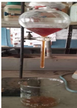
Figure 3: Separation of biodiesel from glycerol
