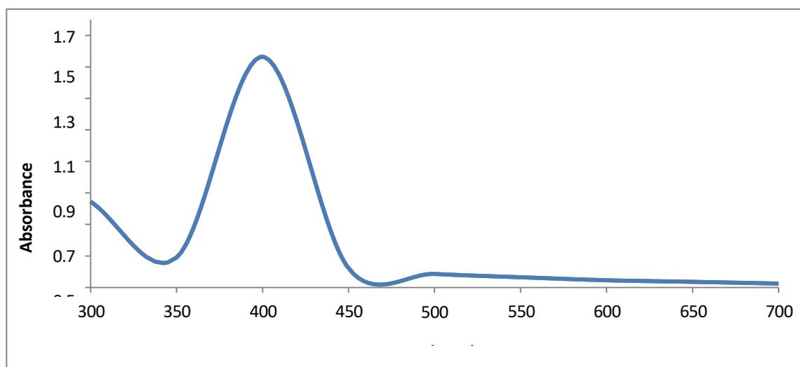
Fig 2. Absorbance spectrum of CuO NPs in ethanol. The spectrum was acquired on a Jenway 6705 UV-vis spectrophotometer in a 10 mm path-length quartz cuvette with ethanol as reference.
