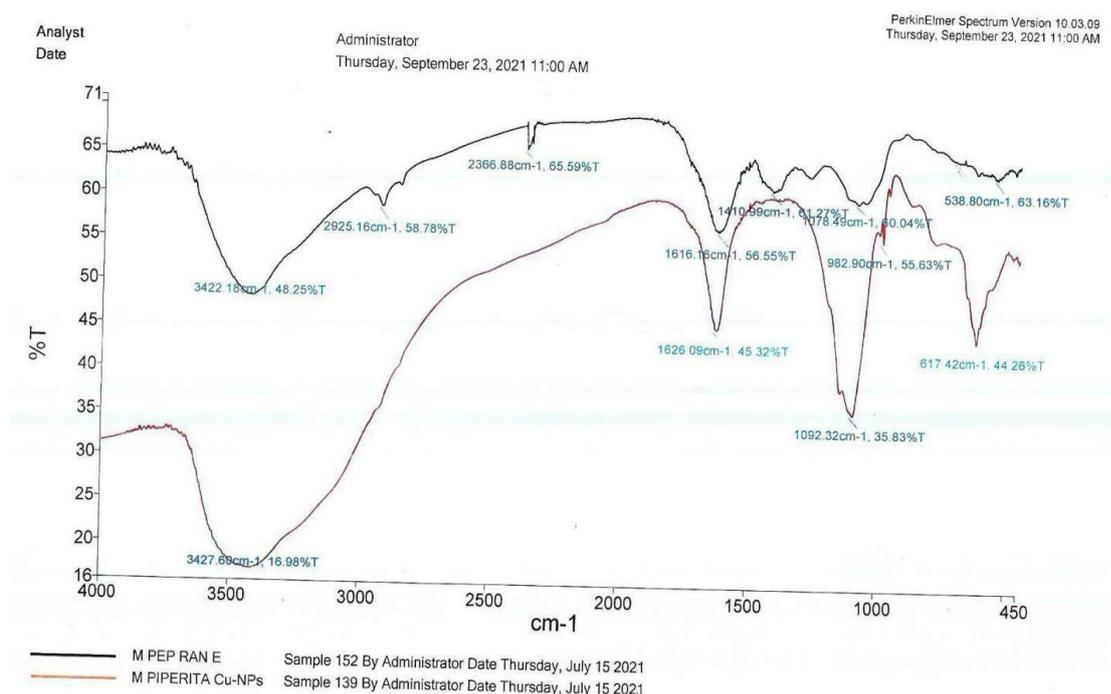
Fig. 3. FTIR spectra of CuO NPs and *M. piperita* leaf extract.
