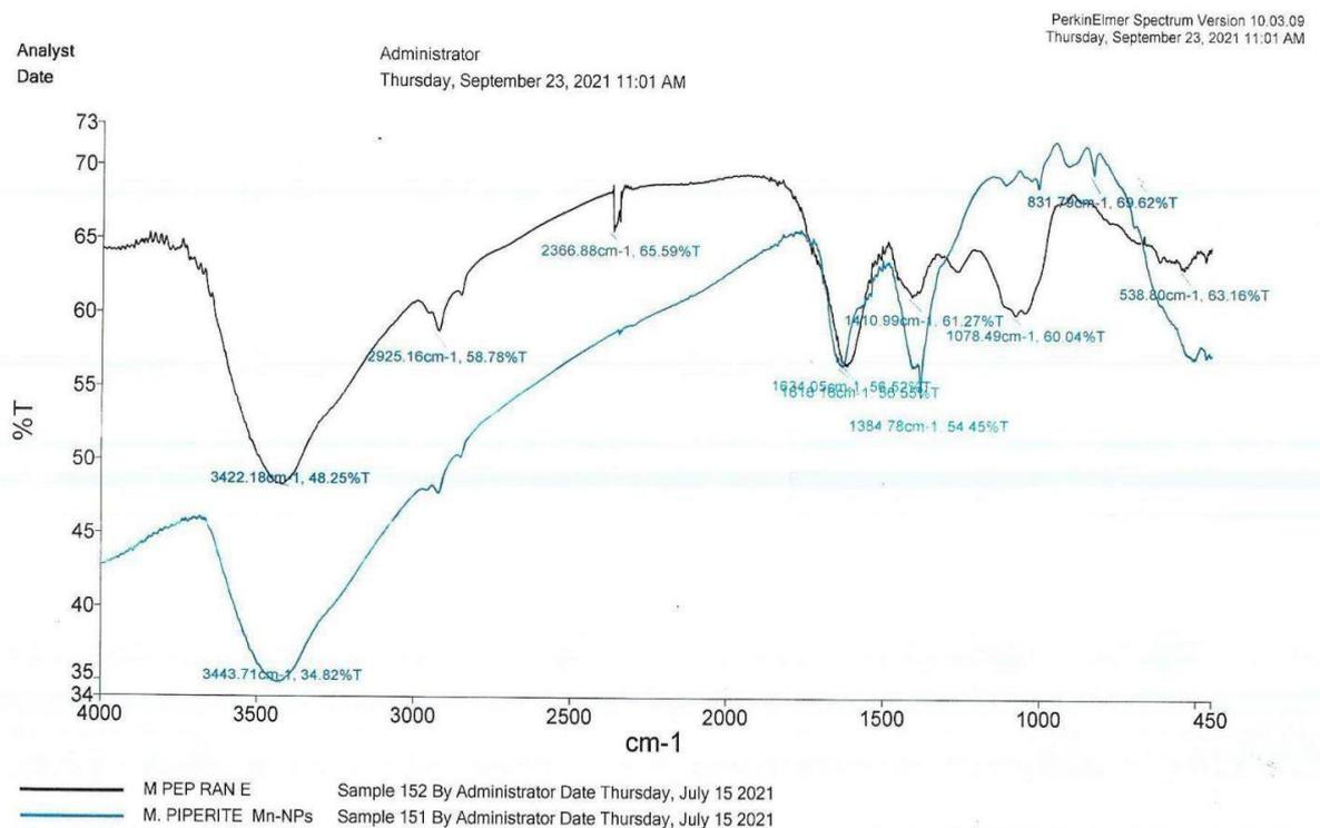
Fig. 4 Showing the FTIR spectra for Mn0 NPs and Plant Extract
