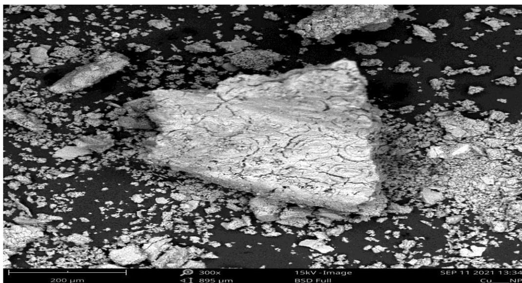
Fig: 5 showing SEM result for CuO NPs
