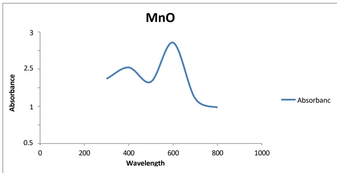
Fig 1: U.V. Absorbance spectrum of MnO NPs in ethanol. The spectrum was acquired on a Jenway 6705 UV-vis spectrophotometer in a 10 mm path-length quartz cuvette with ethanol as reference.
