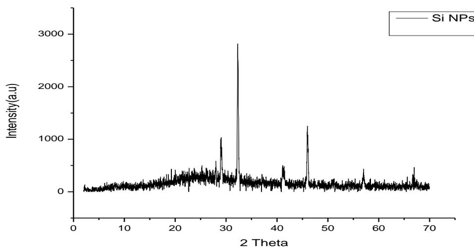
Fig 3. X-Ray Diffractometer Spectrum of the Synthesized Si-NPs
