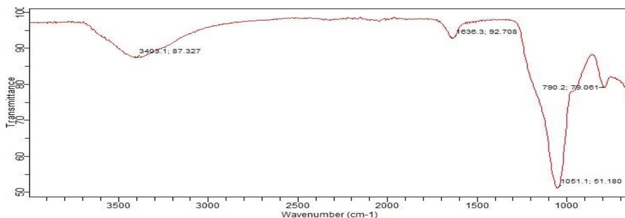
Fig 2. Fourier Transformed Intra-red Spectrum of Si-NPs
