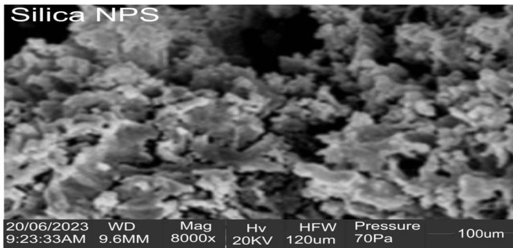
Plate 1. Scanning Electron Microscope Image of the Si-NPs at 8000×Mag
