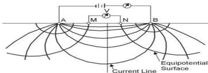
MN = Potential electrode spacing and AB = Current electrode spacing
