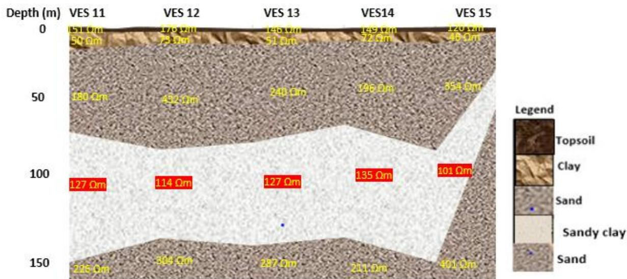
Figure 7: Geoelectric sections of VES 7-15 obtained from the study area. In VES 15, the sandy- clay formation layer thickness is small compared to other parts of the study area. The second aquifer in the vicinity of VES 15 is susceptible to contamination due to its proximity to Earth surface.
