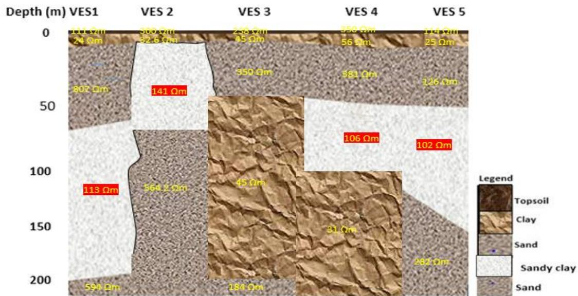
Figure 5: Geoelectric sections of VES 1-5 obtained from the study area. The fifth layer at VES 4 station is a clay formation, and this part of the study area is not suitable for siting of boreholes except if the borehole will be drilled to a depth greater than 200 m below the ground surface.
