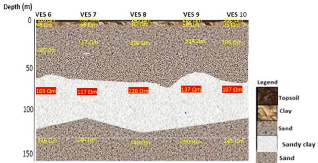
Figure 6: Geoelectric sections of VES 6-10 obtained from the study area. The second aquifer is overlain by a thick sandy-clay formation which protects it from contamination.
