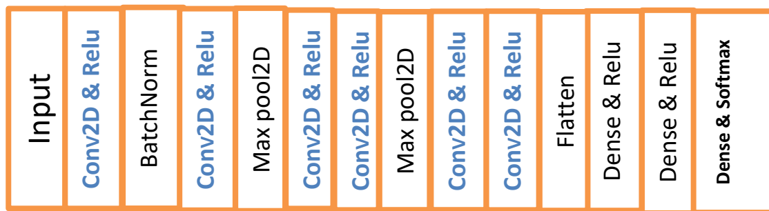
Figure 2. Illustration of the final network architecture of our Proposed CNN model
