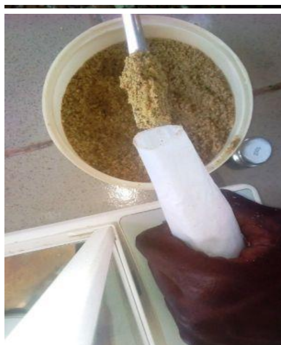
Plate 4. Introduction of sample into thimble
