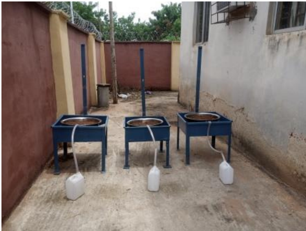
Plate 3: Complete Lysimeter set up
