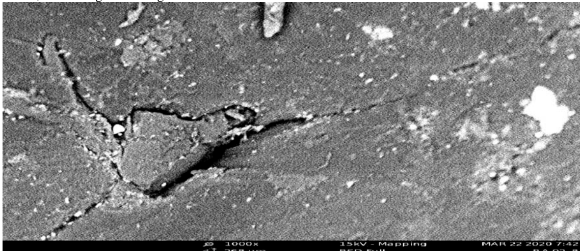
Plate II: SEM micrograph of 8 % wt PA reinforced PVC composite at X1000 magnification
