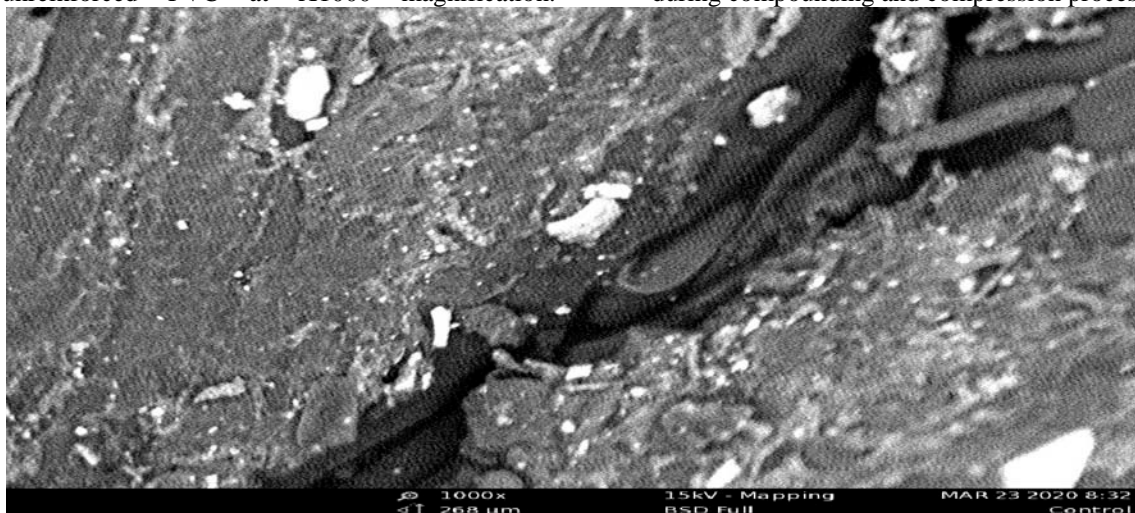
Plate I: SEM micrograph of pure PVC at X1000 magnification
