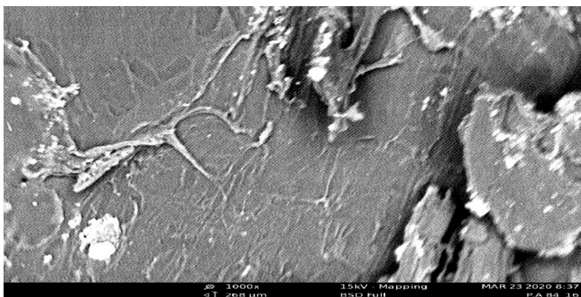
Plate III: SEM micrograph of 12 % wt PA reinforced PVC at X1000 magnification
