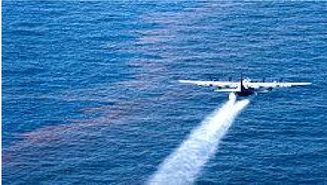
Fig.8. A C-130 Hercules drops an oil-dispersing chemical into the Gulf of Mexico
