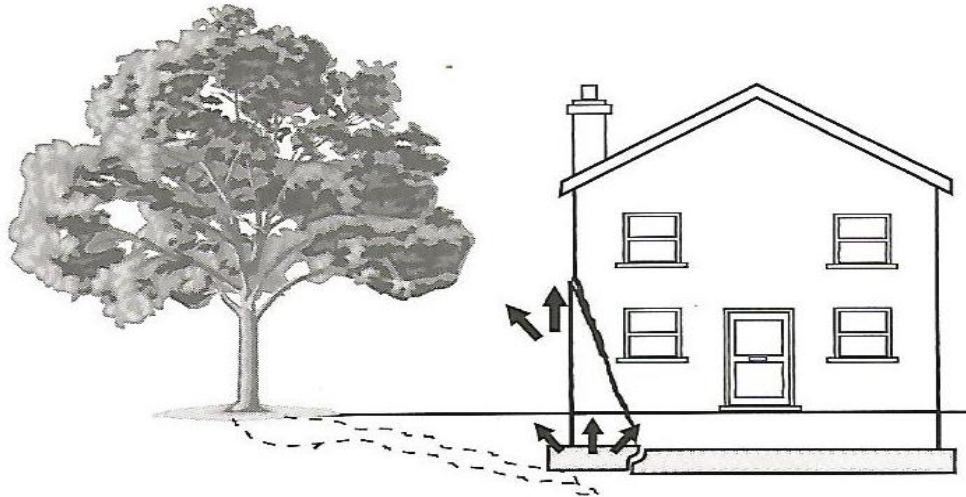
Fig. 1 -Root growth expands. It applies pressure upwards and outwards on sub-soil and building
