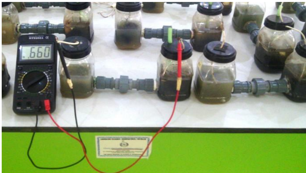
Figure 1. Designed Double Chamber Microbial Fuel Cell (MFC)
