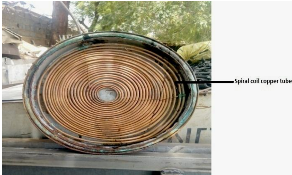
Plate (III): Spiral coil receiver- absorber insulated with glass fibre
